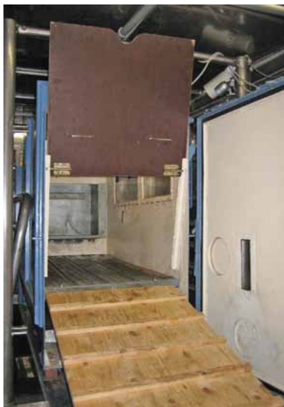
Plate 8: Opened pig chamber with ramp for driving the animals into the chamber.
