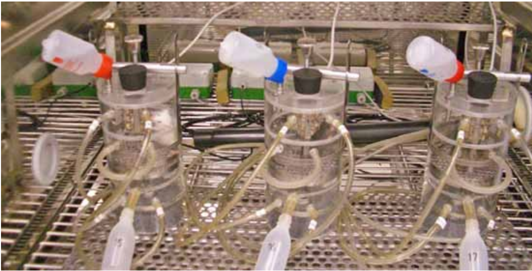
Plate 9: Mice chambers equipped with water flasks and urine collecting bottles.
