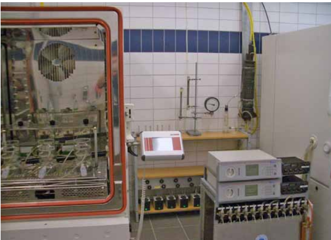
Plate 10: Mice chambers in the climatization closet (left) and gas analyzers (middle) and airflow meters (right).
