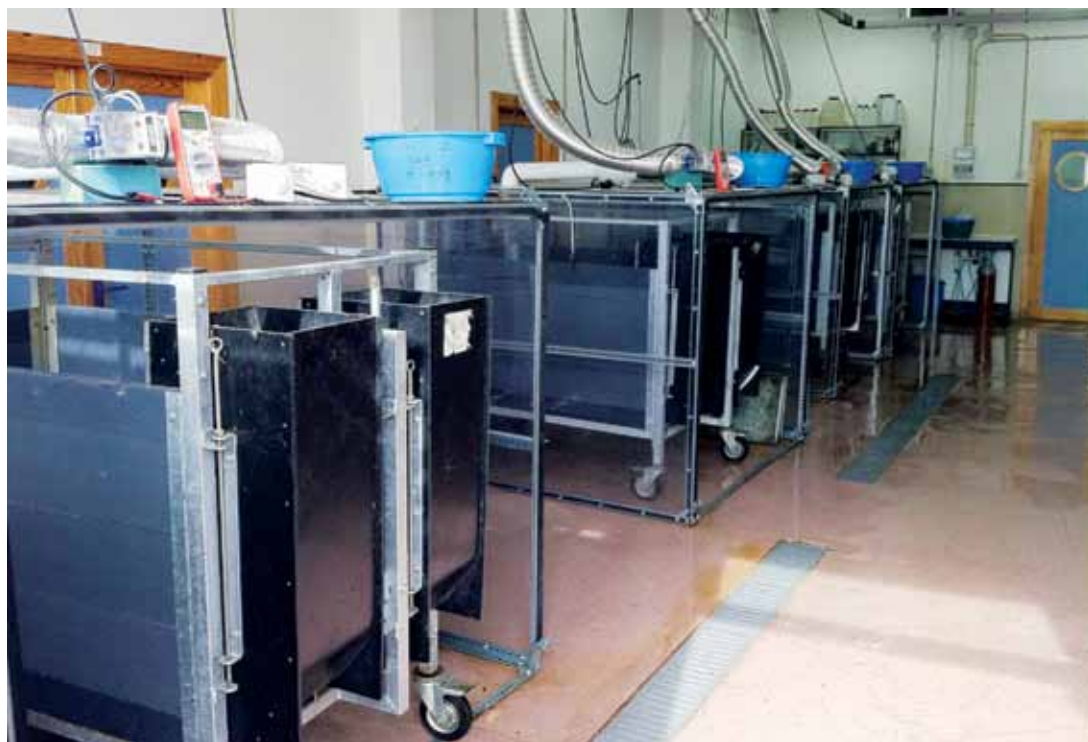
Plate 2: CSIC sheep and goats respiration facility composed of chambers and crates to hold the animals.
