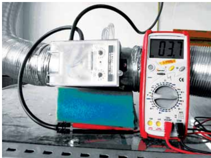
Plate 7: Top of the chamber at CSIC showing the flow meter and electronic measuring unit.
