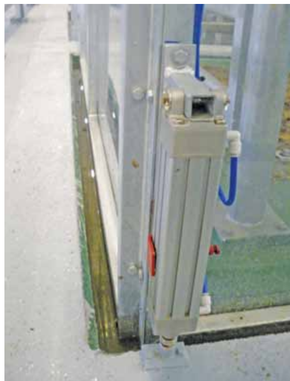
Plate 3: Pneumatic rams fitted one to each corner of the chamber, which lift the entire chamber from the water filled recess used to seal it. Lifting the chamber is initiated by a button on the chamber or automatically if the power fails or oxygen concentration decreases below 18%.
