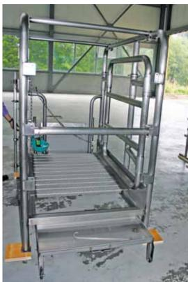
Plate 5: Existing metabolic crate for sheep. The feeding and water trough can be seen in the front. Urine and faeces are collected separately beneath the crate.
