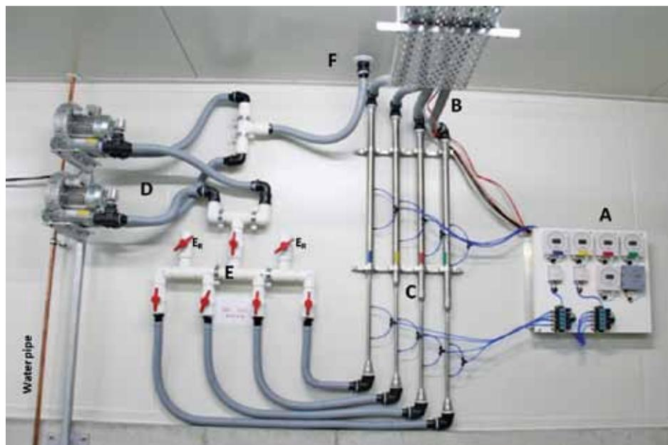
Plate 11: A dedicated gas switching unit (middle) and a gas analyser (bottom) are allocated to a system of eight chambers (sheep). A diaphragm pump (close to the gas switching unit) supplies the sample to the gas analyser, but the sample is split into two streams using a sample conditioning (top), one for  $\text{CH}_4$ ,  $\text{CO}_2$  and  $\text{H}_2$  and another for  $\text{O}_2$ .
