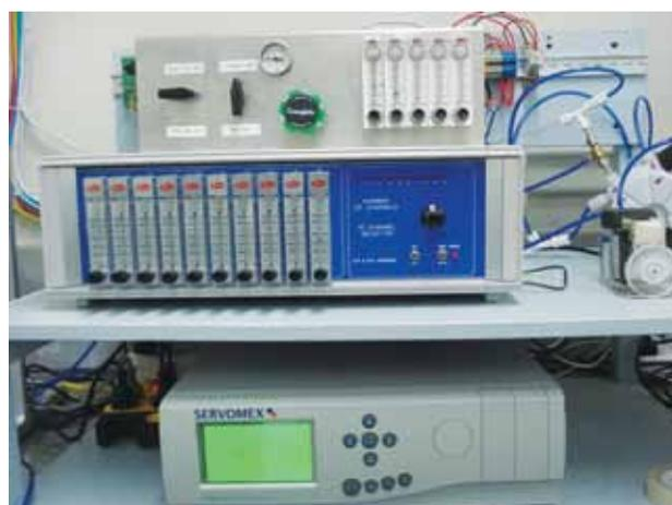
Plate 12: Sample drying system. Sample is delivered ( $\sim 2$  L/min) to the analyser using a micro pump (F), but is first dried using a heated drier (D) and then a non-heated drier (E). Removal of moisture from the sample requires dry air to be circulated in counter flow (4 L/min) to sample. Dry air is generated by a self-regenerator drier (C), but to avoid condensation, a refrigeration unit (B) is placed between the pump (A) and the dry air generator (C).
