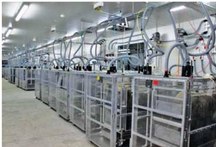
Plate 2: The sheep facility comprises three independent systems. Each system integrates eight respiration chambers. The diagram shows a single system with eight chambers and the configuration of pipes for gas flow, manifold for adjusting flow, sampling lines, data acquisition, sample conditioning, etc.
