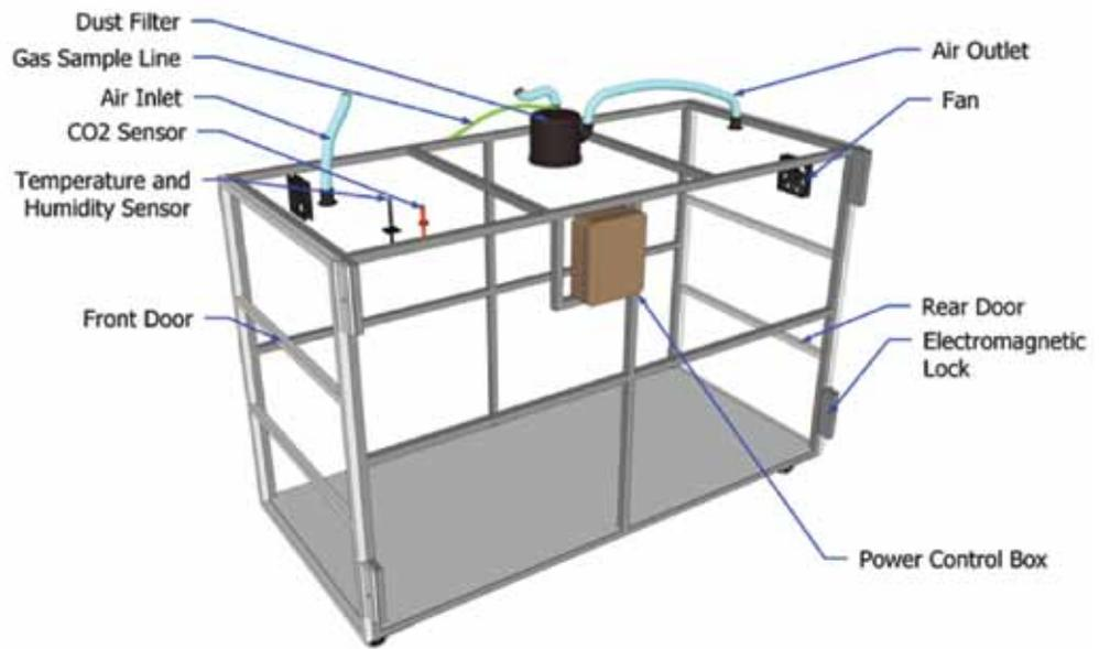
Plate 4: A modified metabolic crate used to hold the sheep in the respiration chamber.
