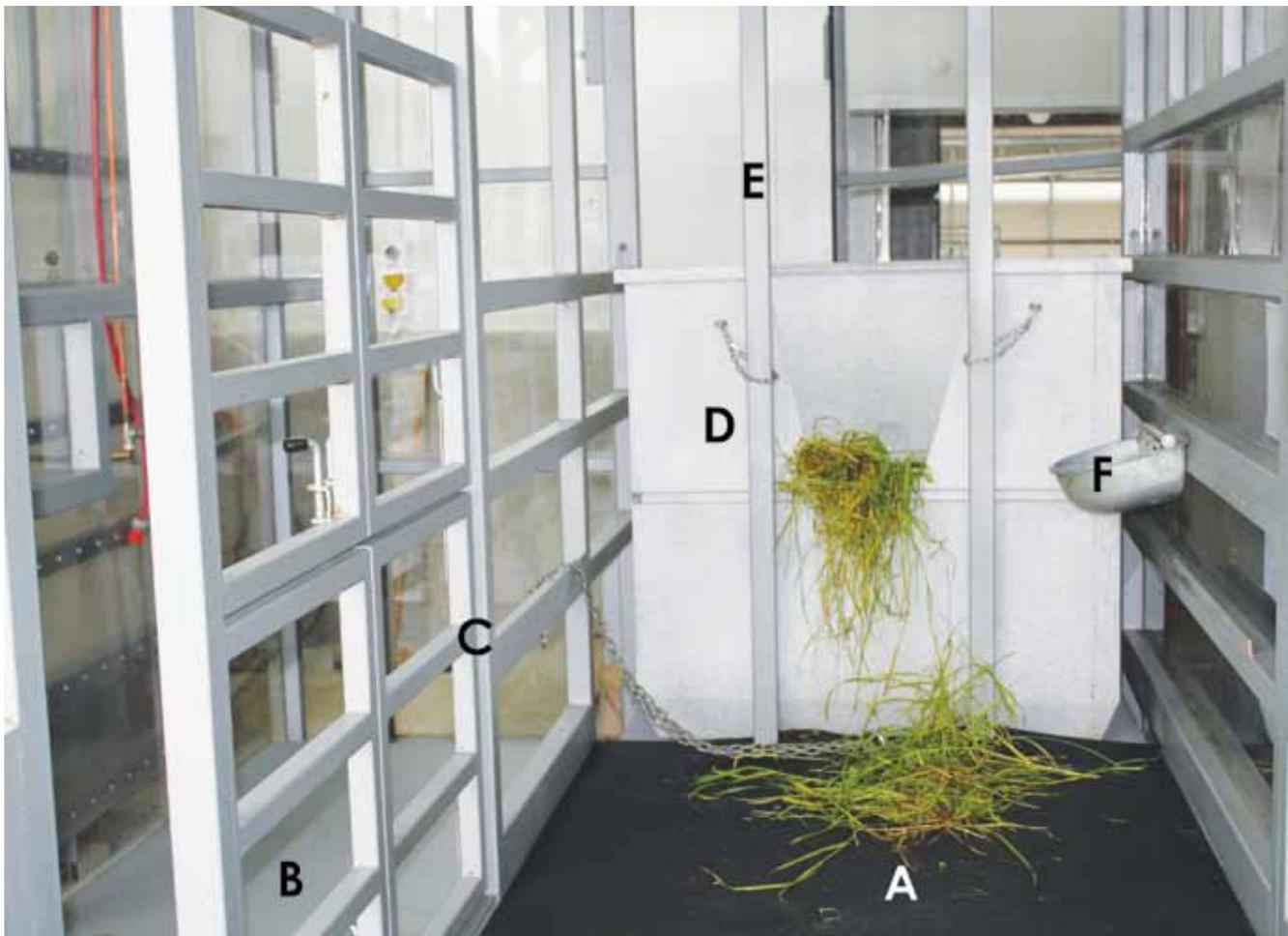
The two rear doors are hinged on either side of the chamber (Plate 14). The main rear door (115 cm wide × 215 cm high) located at the right side is used for animal access, whereas the smaller door (90 cm wide × 215 cm high) located at the left side is used for operator access. These doors are secured with three large clamping wing nuts ensuring that an air-tight seal is achieved by the door against the main chamber frame.
