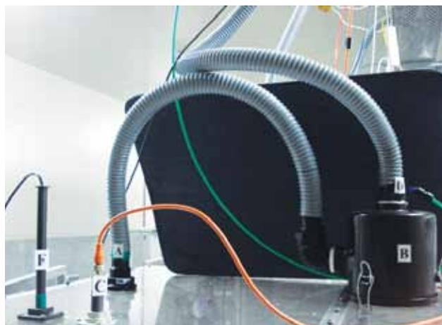
The air handling capacity of each pump is about 1230 L/min, but regulation of air flow is based on two sets of four chambers (Plate 10) and there is a common air flow manifold and pumping system for each set. The pumping system for each set of four chambers involves two pumps connected in parallel (Plates 2, 10).
