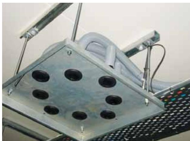
Plate 9: Top of the chamber showing the ducting for air to leaving the chamber via outlet (A), before it is filtered (B) and sampled (D) to determine gas concentrations. The chamber is fitted with a temperature and humidity sensor (F) as well as a CO<sub>2</sub> concentration monitoring sensor (C).
