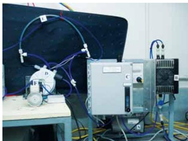
flow rate. The dry air is provided by a heatless self-regenerative air drier (Nexus Analytical Pty Ltd, Australia). Room air supply to the dry air generator is via a Thomas 617CD22-194C pump (Thomas, Sheboygan, WI, USA). However, to avoid condensation inside the tubing supplying air from the pump, the air is cooled to 4°C using a thermoelectric refrigeration unit (XC3000A, Tropicool, Christchurch, New Zealand).
